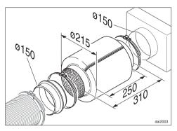
To achieve even further reductions in noise levels, a special silencer can be fitted in the ducting system...
